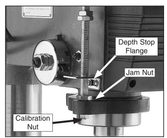
Figure 41. Depth stop assembly.
